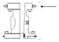
A. The leak can be easily repaired by removing the bolt and changing the packing gland
